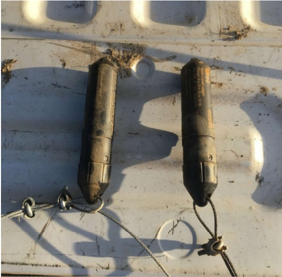
Figure 12. Pressure transducers with data loggers ready for installation.
